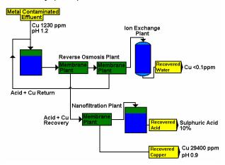
Heavy metal removal/ recovery is particularly important in the metals industry across a range of sectors from mining tailing ponds to processing applications. Esmil membrane technology is well suited to solving the problem of heavy metals due to the high rejection efficiency by the membrane materials. This can reduce the load on current conventional treatment systems such as ion exchange or act as a standalone plug and play system to achieve the desired effluent qualities.
