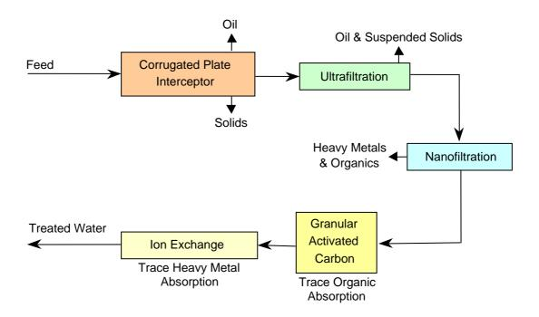
Figure 1. Esmil Produced Water Treatment Plant Schematic
