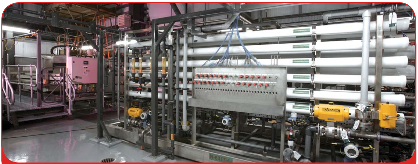
The photo shows the Produced Water Ultra-filtration and Nano-filtration Membrane Skid, with Filter Press to the left.
