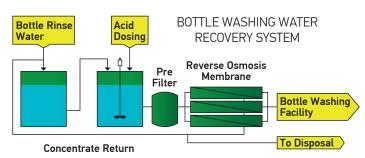
water contains high levels of soluble organics (COD), from the washing of dirty soft drink or alcoholic beverage bottles. RO membranes remove organics, hardness and bacteria from the water enabling optimum recovery to the washing facility.
