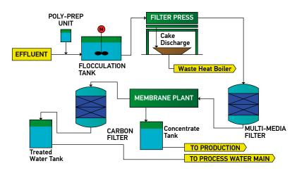
**Permeate** for use as general site process water or boiler feed
