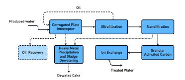
The oil and suspended solid free water is treated using membrane Nanofiltration, which removes the bulk of heavy metals and organic compounds. Trace organics and heavy metals in the Nanofiltration permeate are removed by **Activated Carbon** absorbers and selective **Ion-Exchange** resin. The pre-treatment by Nanofiltration significantly increases the bed life of these two media...
