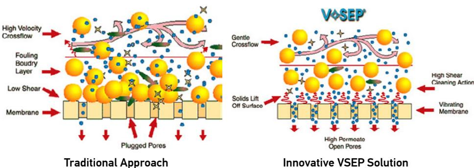
The high shear processing exposes the membrane pores allowing for maximum permeation of treated water. The contaminants and a portion of the water are rejected by the membrane and remain on the concentrate side. This 'concentrate' will contain the vast majority of pollutants from the feed and therefore can potentially be sent to Evaporation Pond, Evaporator or Reapplied to the landfill.
