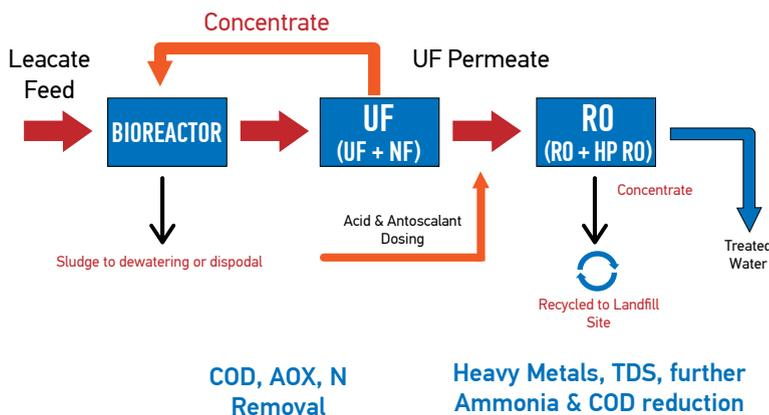
The first stage in our Leachate treatment process is the Biological Process where microbes are used to degrade pollutants that are then filtered by a series of UF membranes in the second stage. Permeate is then treated using RO membranes to produce water suitable for reuse or discharge to the local sewer. The key property of effluent is its biodegradability or COD/BOD ratio.
