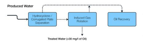
Conventional Treatment involves Hydrocyclones / Corrugated Plate Separation followed by Induced Gas Floatation and Media Filtration to remove oil and suspended solids below 10-30 mg/l limit. The treated water is suitable for on board discharge or for reinjection purpose.
