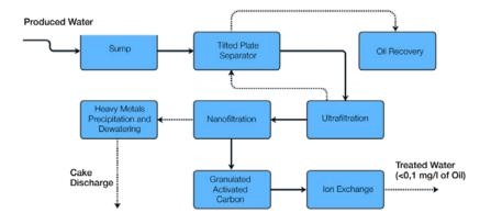
Ultrafiltration reject stream is recycled to the front end of the process and the concentrated oil is reclaimed on site from TPS unit. The various sludge and aqueous waste streams from the main process are combined before undergoing precipitation, flocculation and filtration, to produce a 'cake' for landfill, and a filtrate that can be recycled through the process.
