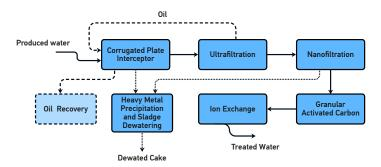
The oil and suspended solid free water is treated using membrane **Nanofiltration**, which removes the bulk of heavy metals and organic compounds. Trace organics and heavy metals in the Nanofiltration permeate are removed by **Activated Carbon** absorbers and selective **Ion-Exchange** resin. The pre-treatment by Nanofiltration significantly increases the bed life of these two media.
